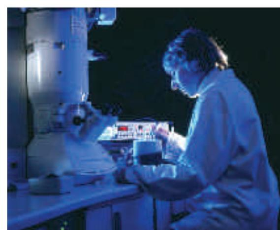
*Scientist preparing a sample in liquid nitrogen before examining it on a transmission electron microscope.*
